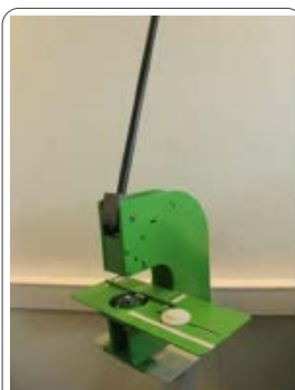
Eyeletting machine Type 66 Handmatig 300/uur
